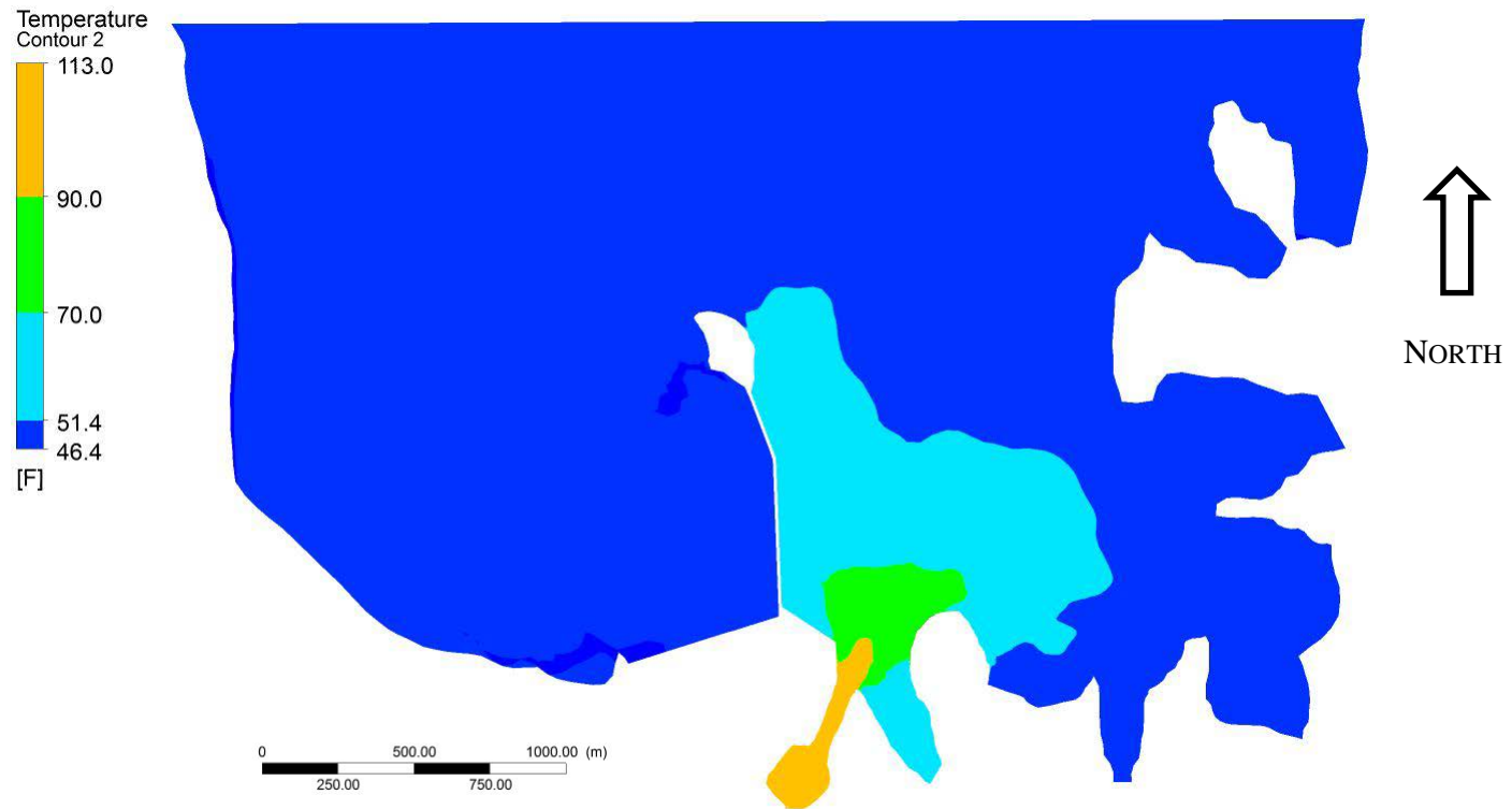
Figure 4. Scenario 4: Winter - High Water; FPSF Generating (Discharging from Reservoir).
